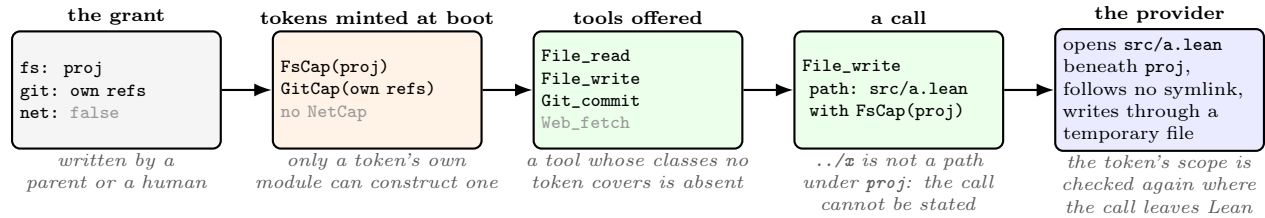
Figure 7: From grant to system call, for a child with one project worktree and no network. The grant decides which tokens exist, the tokens decide which tools the model is offered, and each call carries its token to the provider, which checks its scope again.
